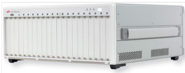
Figure 6. M9018A 18-slot chassis.
