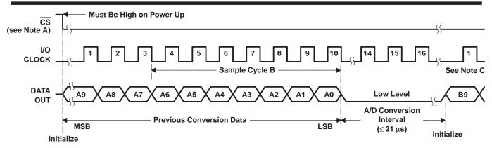
Figure 9. Timing for 16-Clock Transfer Not Using CS (Serial Transfer Completed Within 21 μs)
