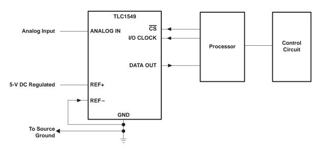
Figure 13. Typical Serial Interface
