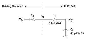
V<sub>I</sub> = Input Voltage at ANALOG IN
