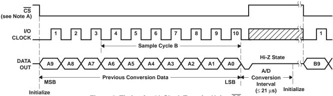
Figure 6. Timing for 10-Clock Transfer Using CS
