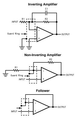
Figure 29. Typical Connections of Guard Rings
