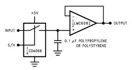
Figure 32. Low-Leakage Sample and Hold
