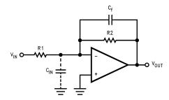
Figure 25. Cancelling the Effect of Input Capacitance
