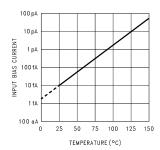
Figure 2. Input Bias Current vs Temperature
