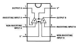
Figure 1. 8-Pin PDIP/SOIC **Top View**
