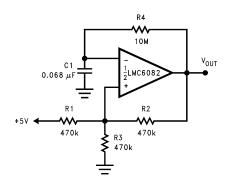
Figure 33. 1 Hz Square Wave Oscillator
