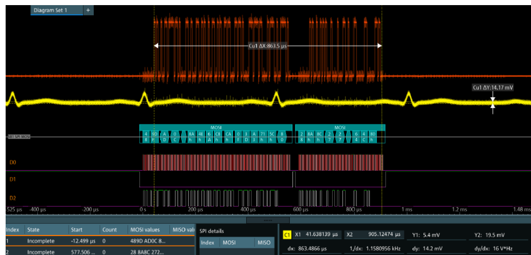
Figure 13-3: Decoded and binary SPI signal
