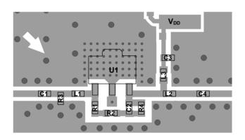
The bias current can be adjusted to support lower noise figure and lower power consumption by removing external bias resistor R4 and replacing R3 as detailed below.
